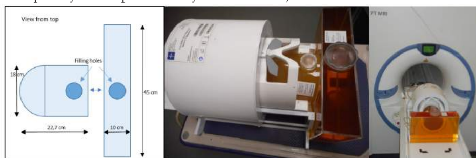
Figure 2: Prototype of the GUFU phantom used for testing of the QA protocol at four GUFU sites. The head and neck part of the phantom is filled with a PVP water solution doped with NaCl and gelled with Agar. This resulted in realistic dielectric properties compared to the emulated tissue ( \epsilon_r = 55 , C = 0.6 S/m) with proper T2 (60 ms) and acceptable T1 (700 ms) relaxation time constant. The shoulder part is filled with a NaCl-doped PVP solution to simulate the dielectric coil load of the human shoulder and body.
