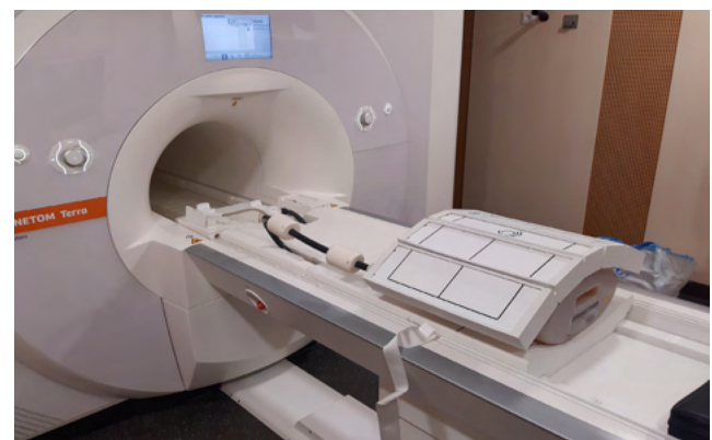
Figure 2: The 8Tx/32Rx ^1\text{H} body array coil designed by Tesla Dynamic Coils installed at the TERRA in Essen.
