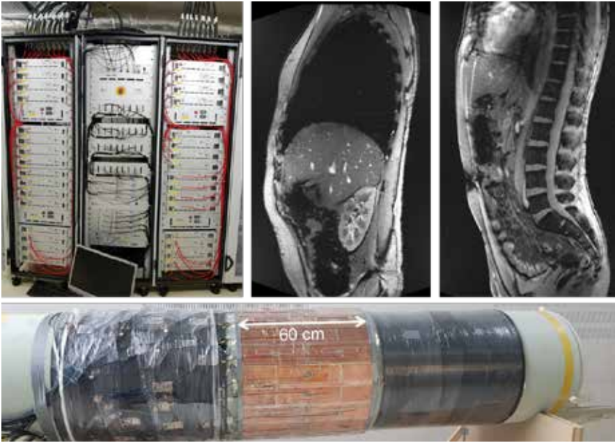
Figure 2. The self-developed 32-channel integrated body coil mounted on the bore liner of the classic 7T at the DKFZ (bottom). The coil is driven by a self-developed pTx system 8 with 32 RF amplifiers, each with 2 kW peak power (top left). First images in two different subjects (top middle and right) demonstrate large field-of-view imaging capability.
